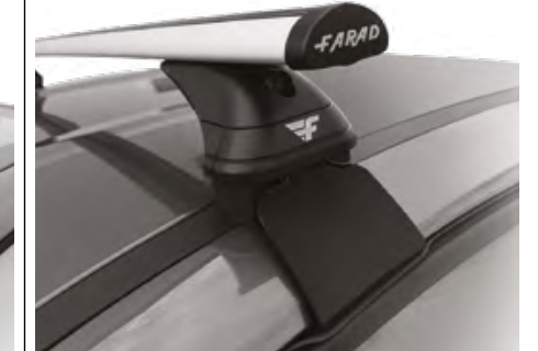
SPECIFIC KIT FOR CARS WITHOUT ROOF RAILS KIT SPECIFICO PER AUTO SENZA CORRIMANO
